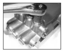
1. With a 22mm socket, remove the three discharge (43) and three inlet (41) manifold plugs.
